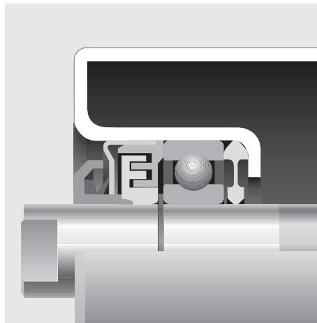
Section through sealing
