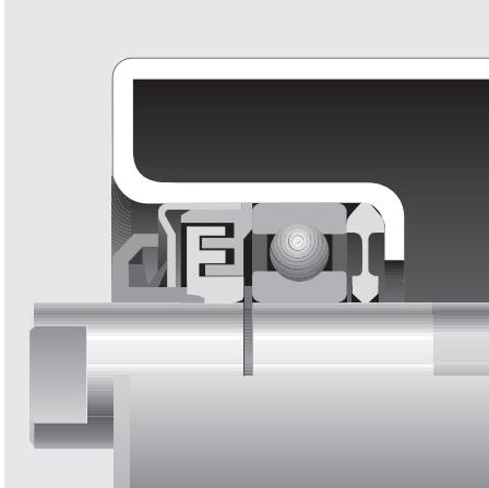
Section through sealing
