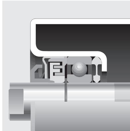
Section through sealing
