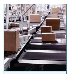
**Transportation – merge and takeaway** Junctions require narrow tolerances and small drum diameters, but they don't have to be problem spots – Schiki Belts 45° angled merge belts are perfect for the job and are also resistant to high temperatures.
