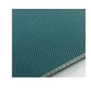
Petrol Green PVC conveyor belt, 74 ShA, 3 plies. Thin, hemispherical, R19 profile allows the best adhesion to the workpiece. Good abrasion resistance.
