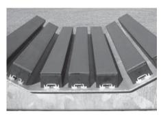
Rulmeca presents a new product to widen the range of components for belt conveyors: impact bars used at the loading point of the conveyor under the hopper. These impact bars utilise the important properties of two materials such as the low friction of polyethylene and a quality rubber to absorb shocks.
