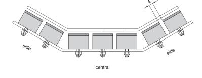
To be used for transoms with 20°- 30°- 35° inclination angle.
