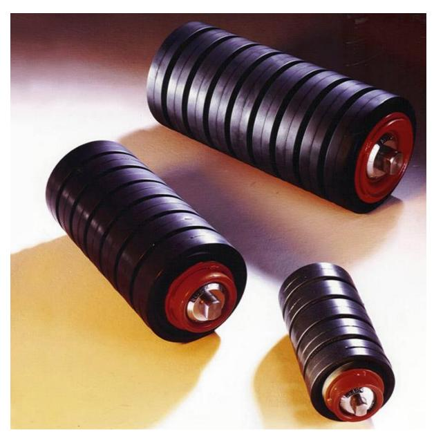
The shock absorbing rollers, more often known as "impact rollers" consist of a base steel roller design, on which are fitted rings, designed to resist and absorb the pressures given by the impact of materials onto the belt.
