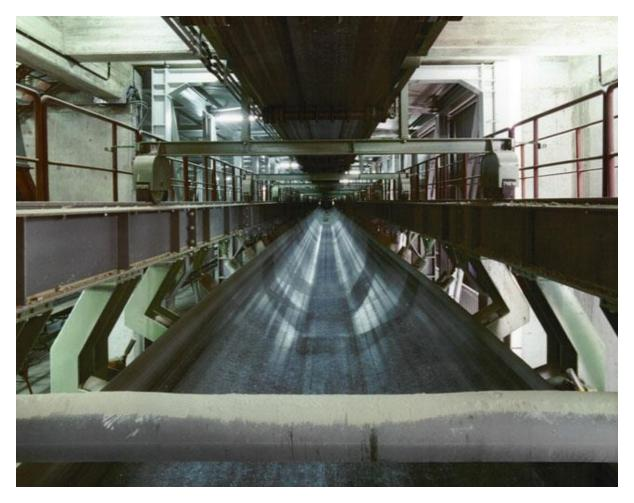
The lower or return sets may also be chosen from varying arrangements according to the requirement: fixed sets with plain steel roller or with spacer rings and suspended sets "garland" with plain rollers and with rings. Transoms and brackets
