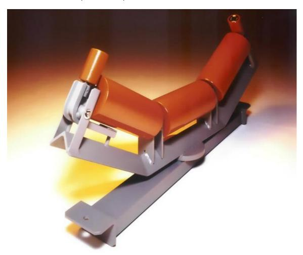
Sometimes the difficult working conditions of the plant results in a lateral movement of the belt. In this case a self-centralising troughing set is used which acts in a way that corrects the belt tracking and maintains it constantly in the central position. The self-centralising troughing set is designed as a series of rollers arranged in a trough positioned onto the supporting transom which itself is fixed to a slewing ring which permits rotation.
