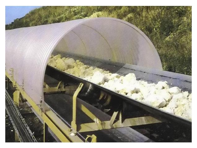
In the project design of a belt conveyor, after having defined the components of primary importance, it is important to consider other accessories such as covers for the conveyor.
