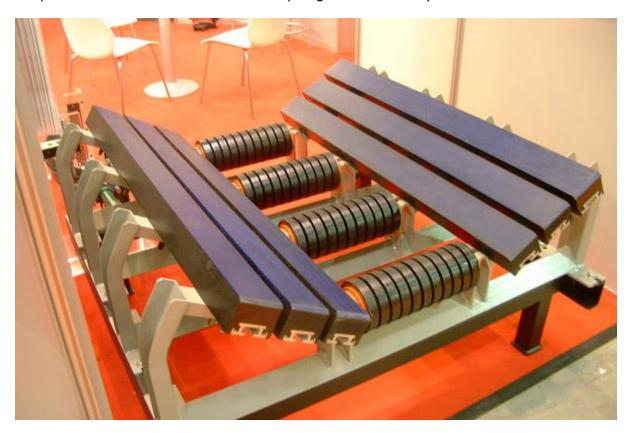
The impact bars, positioned under the loading points of the conveyor, prevent damage to the belt, keep the belt stable and avoid the spillage of the conveyed material.
