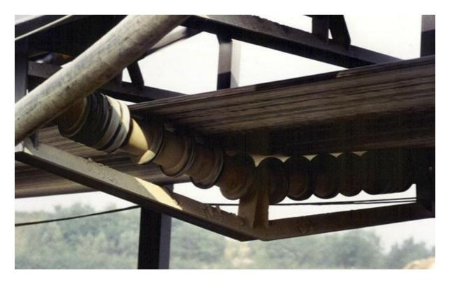
The straight tracking of the belt may be compromised by the type of conveyed material, specially when this material is sticky and thereby adheres easily to the belt surface.
