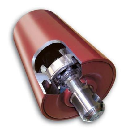
PRECISMECA / RULMECA GROUP Heavy Duty Rollers are designed for heavy duty open mining applications. Thanks to the high quality machined parts and a non contacting multi-chamber labyrinth seal, the rollers run with a whisper. The high quality machining process is a guarantee for a long service life of the PRECISMECA rollers - 8 years in operation 24 hours a day is not a rarity. Return rollers with rings should not be used as belt tensioning devices.
